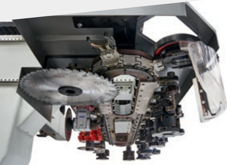
Chain-type tool magazine 22 positions with 180 mm between centres.
